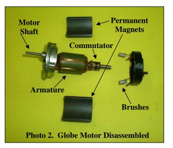
It is useful to consider some relationships between motor torque, speed, and current consumption. As a rule, we will not be concerned with power consumption or efficiency since contest time limits are usually too short for this to be a concern.
