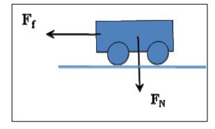
Figure 2. Frictional Forces Diagram
