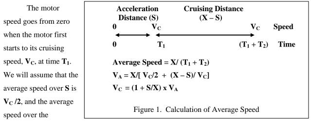
remainder of the distance, X - S, is the constant cruising speed  $V_C$ . The corresponding times are the respective distances divided by their speeds, or
